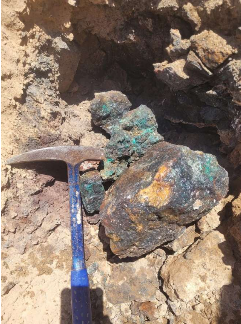
Figure 4: Sample 17397, easting 264520, northing 8065874, quartz vein zone with specularite, CuOx – malachite and chalcopyrite. Cu 4.92%, Au 2,47 g/t
